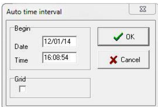
It is important to take care while formatting the fields. The date (DD/MM/YY format) and time (HH:MM:SS) must have 2 characters (e.g. 01:58:09 08/01/14 = correct; 1:58:9 8/1/24 = wrong). Clicking on the grid check box displays a grid.
