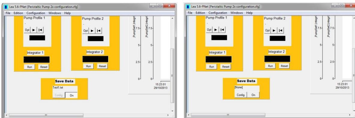
To **stop saving** the data click the *On* button once again, and **[None]** will be displayed at the top. If data storage is stopped, it is impossible to save further data.
