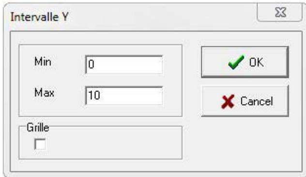
The minimum value must be smaller than the maximal value. Clicking on the grid check box shows a grid.
