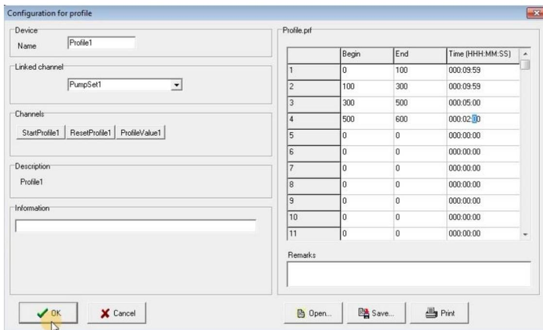
Flow profiles up to 50 steps can be entered, saved as a file and printed out.
