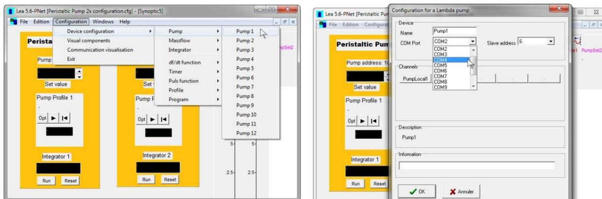
Set address of the pump (refer to [http://www.lambda-instruments.com/?pages=peristaltic\\_pump\\_preciflow\\_remote\\_control#pc-control](http://www.lambda-instruments.com/?pages=peristaltic_pump_preciflow_remote_control#pc-control) for the pump address).
