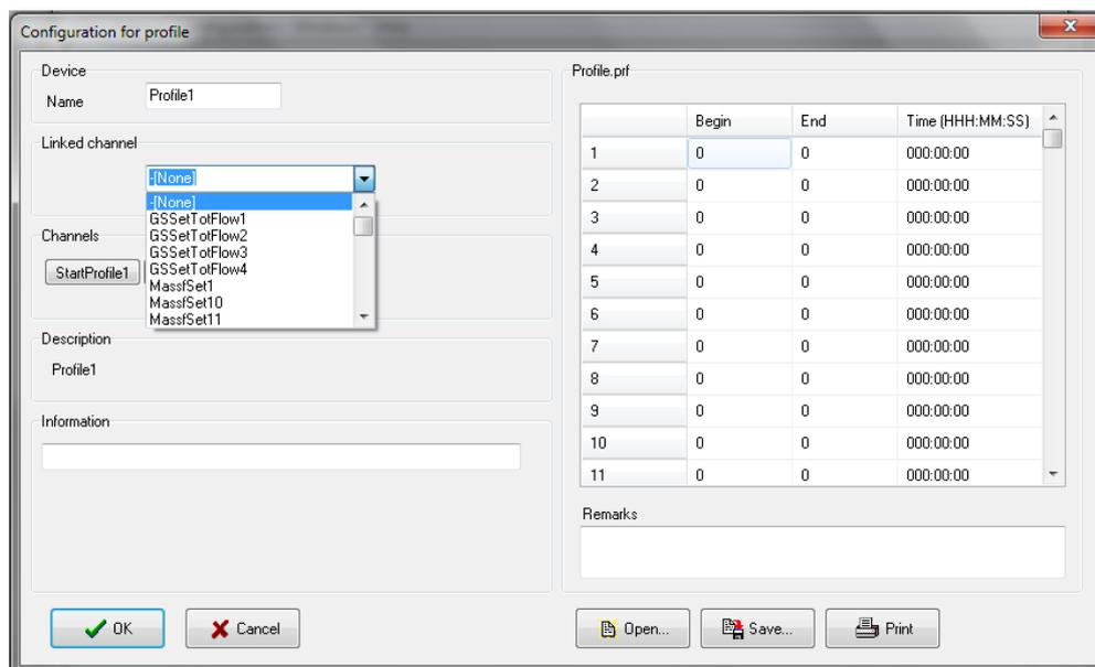
Enter the 'begin' and 'end' values and the duration. The format for duration must be correct: use three figures for hours and two for minutes and seconds respectively. If the duration is set to zero the segment will be ignored.
