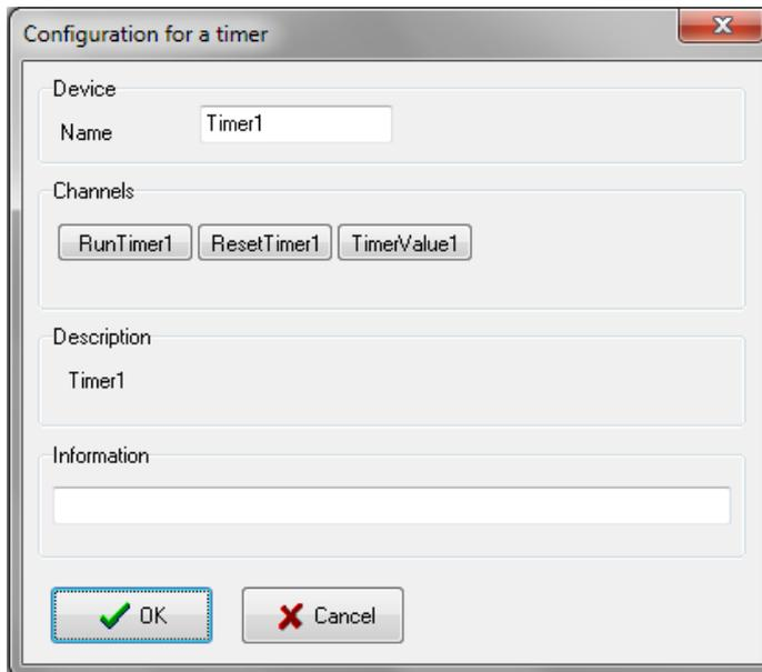
The channel buttons allow each channel to be individually configured. The Description field displays the internal device name. The Information field is free for user input.
