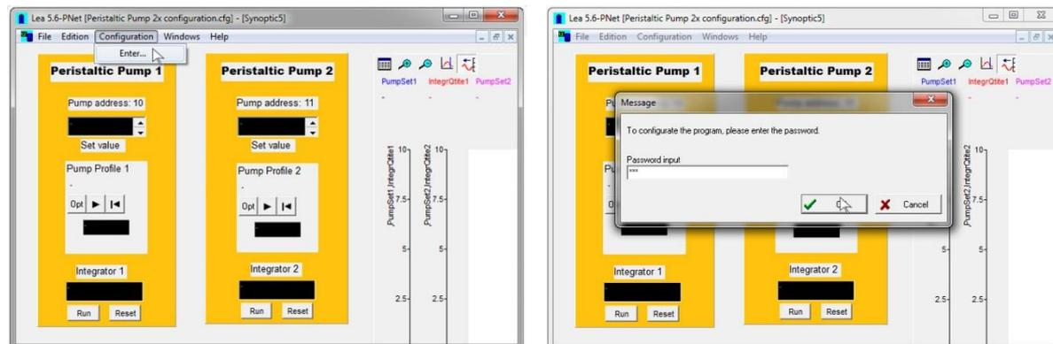
In the menu *Configuration*, select *Device Configuration*, *Pump* and click on *Pump1*.
