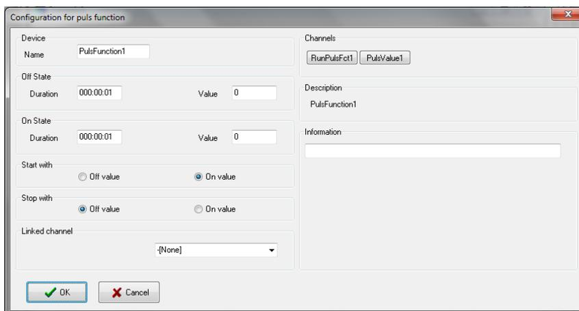
The channel buttons allow each channel to be individually configured. The Description field displays the internal device name. The Information field is free for user input.
