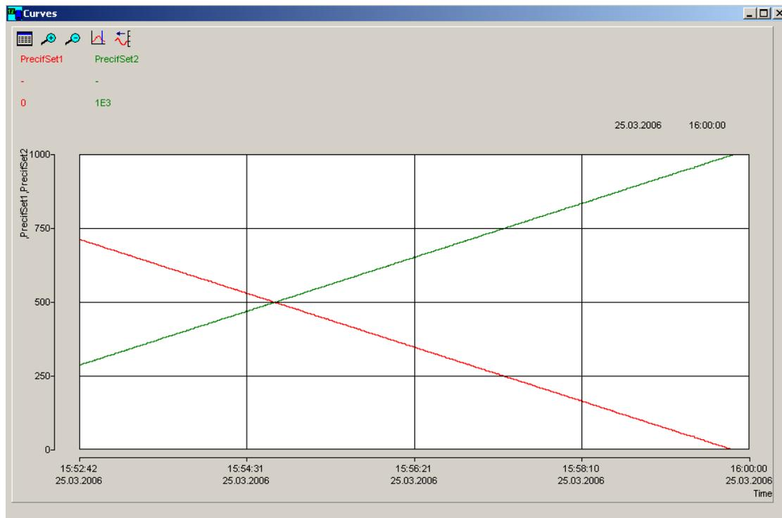
Curves showing the set points of the controlled pumps as a function of time.
