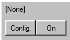
To save channel values to a text file, click on the *Config.* button to open the 'Save data to text file' window. Select the *File* tab and enter the *file name* and select the destination to save the file.
