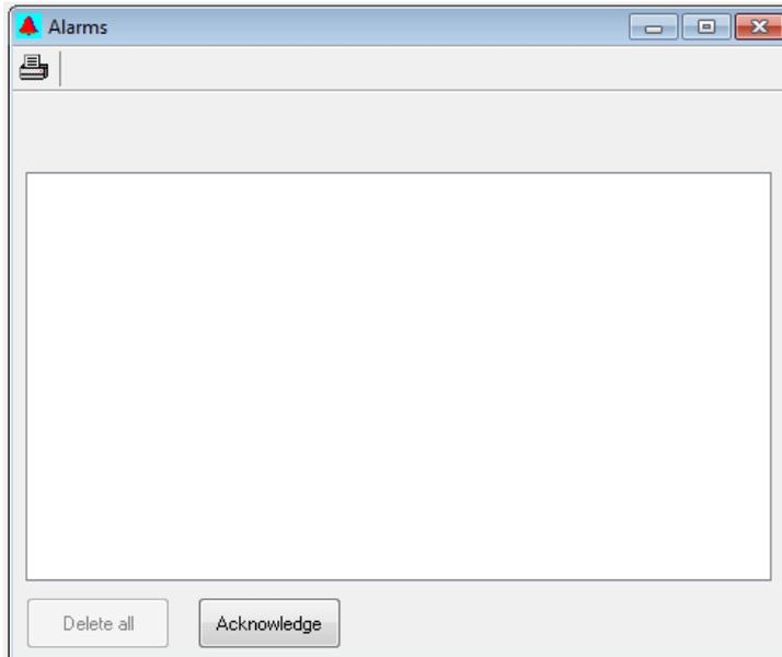
When an alarm is triggered the date, time, channel name and value are automatically entered into the alarm list. To cancel an acoustic alarm, press the *Acknowledge* button.
