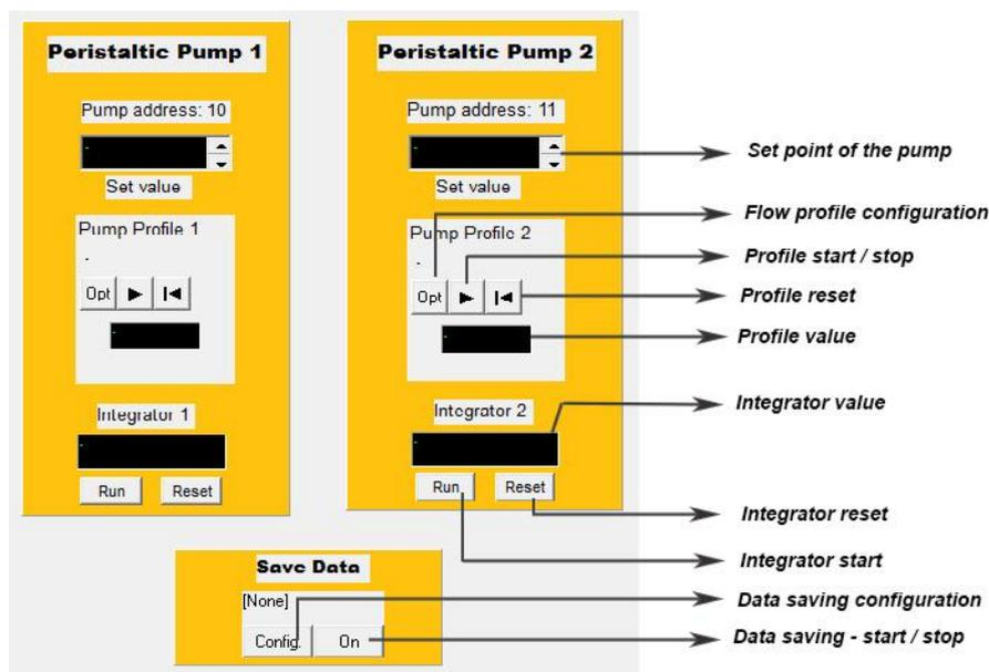
To enter a new set point value of the pump click on the input field. A second field is displayed into which the new target value can be entered. Press the *Enter* key to confirm the entry. If the value is outside the calibration limit, it will not be accepted by the system.
