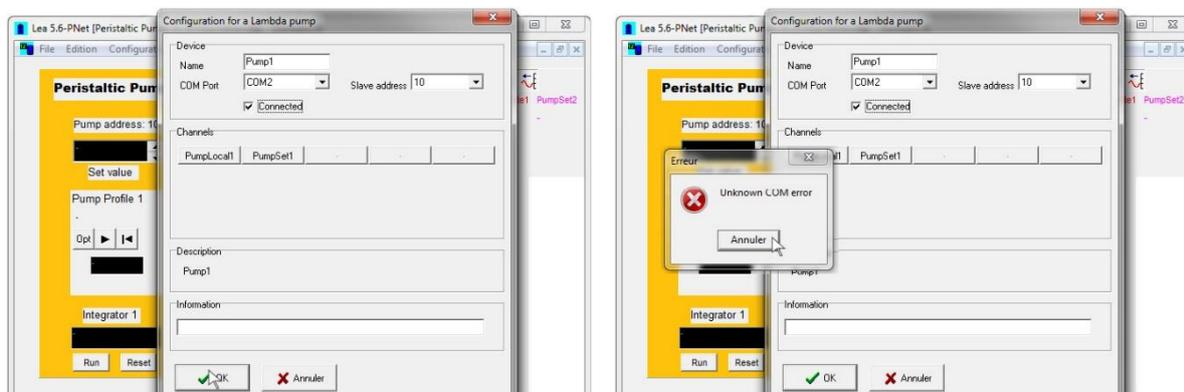
The *Description* field displays the internal device name. The *Information* field is free for user input.
