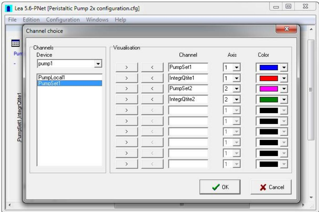
Select a channel from the list, copy it into a field in the channel column with the '>' button. Choose an axis (Y1 and Y2 are displayed on the left, Y3 and Y4 are displayed on the right). Select a colour from the colour list. To delete a channel click on the '<' button.
